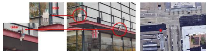
Fig.1 Lidar based monitoring solution connected to an RSU to share data with connected vehicles
