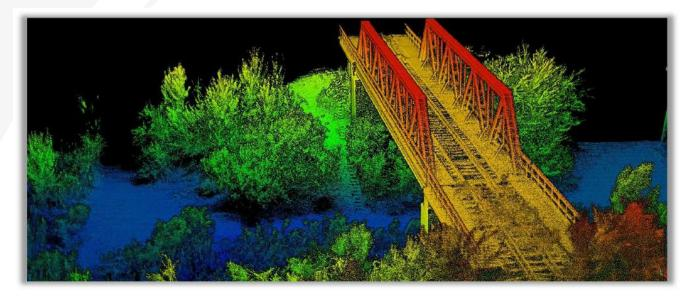
This road survey was produced using a Velodyne VLP-16 LiDAR sensor alongside an OxTS Survey+ INS. The data was processed using OxTS Georeferencer.
