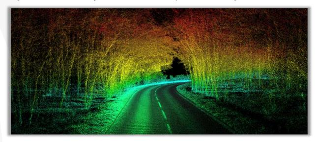
The below street survey was produced using a Velodyne VLP-16 LiDAR sensor alongside an OxTS xNAV v3 INS. The data was processed using OxTS Georeferencer.
