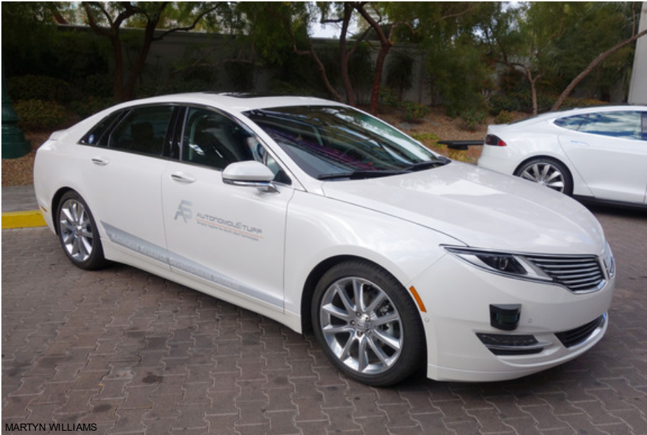
A Lincoln MKZ modified by AutonomouStuff with additional LIDAR sensors on the front bumper, shown at CES in Las Vegas on Jan. 7, 2016.
