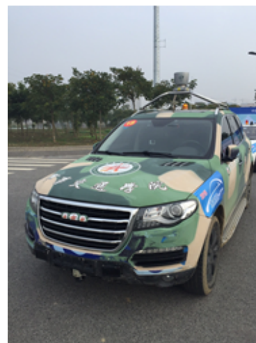
Velodyne LiDAR-equipped vehicle from the recent Intelligent Vehicle Future Challenge in China
