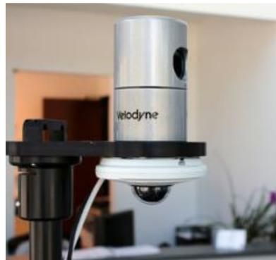
Combining Velodyne's real-time 3D LiDAR with PZT camera for security and surveillance purposes.
