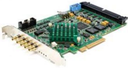
Gigabits/Second (Gb/S). Simultaneously, control commands and triggers can be sent to the camera 20 Mb/S (with a trigger accuracy of +/- 2 nanoseconds). Up to 13 W of power can also be supplied to the camera. All this happens over a single piece of industry standard 75 Ohm coaxial cable. Multiple CXP links can be aggregated to support higher data rates (e.g. four links provide 25 Gb/S
