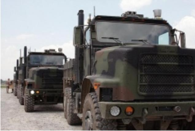
Sensors and cameras are seen atop two autonomous, unmanned Cargo UGV trucks that are part of a larger convoy that also includes human-driven vehicles in a test of robotic systems at Fort Pickett, Va., on July 30, 2012.
