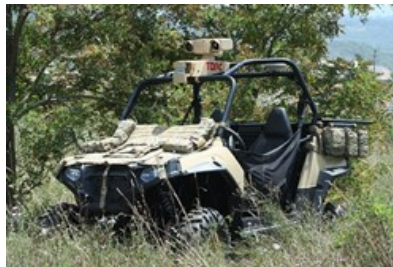
Velodyne's HDL-32E LiDAR real-time LiDAR sensor for object detection and collision avoidance mounted on TORC's robotic vehicle. Courtesy of TORC Robotics http://www.torcrobotics.com
