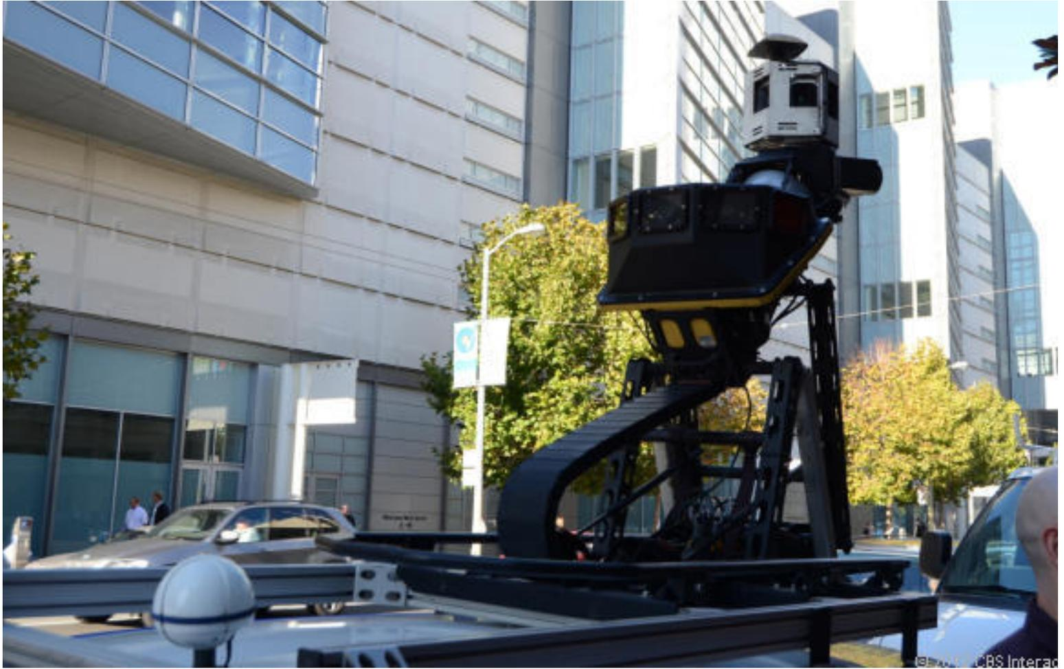
The most obvious bit of acquisition equipment is the camera and Lidar array atop the True car.
