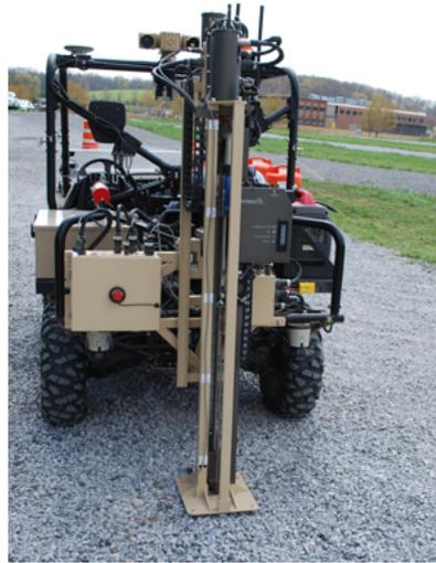
Realizing that the Lightweight Tactical All-Terrain Vehicle (LTATV) model used for prototype development may not be the final solution, it was critical to have a modular, platform-agnostic architecture that would allow for future RAZTEK systems to utilize a different LTATV platform with minimal reconfiguration. The robotic conversion also needed to maintain the ability for manned operation.
