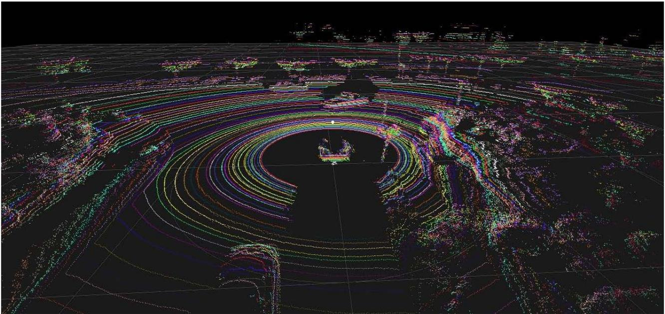
Figure 4. Digital Sensor Recorder Display of HDL-64E Data.
