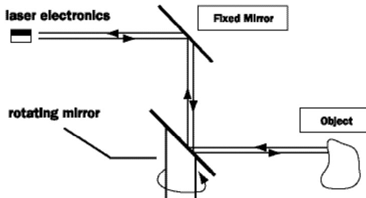
Figure 1. Single emitter/detector pair rotating mirror lidar design.
