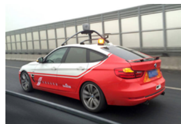
On the roof, Baidu's modified BMW 3 Series sports Velodyne's HDL-64E LiDAR sensor
