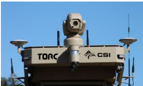
The 360 Degree Situational Awareness System provides full visual coverage for augmented operator awareness
