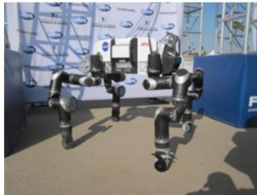
RoboSimian, equipped with Velodyne's HDL-32E 3D LiDAR sensor
