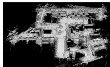
Above and at right, demonstration images of the Real Earth/Velodyne LiDAR solution -- a fast, cost-effective way to create LiDAR-sourced maps without GPS
