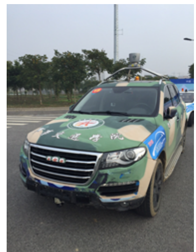
Velodyne LiDAR-equipped vehicle from the recent Intelligent Vehicle Future Challenge in China
