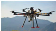
True Reality GeoSpatial Solutions's octocopter, equipped with Velodyne's lightest and most affordable LiDAR sensor, the VLP-16 LiDAR Puck
